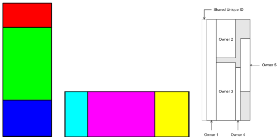
Figure 1: Models for data partitioning. Data subjects are rows, and attributes are columns. Left: horizontally partitioned data - data subjects are partitioned among database owners. Center: Vertically partitioned data - attributes are partitioned among database owners. Right: complex data partition with five database owners.
