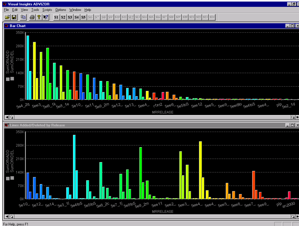
Figure 7: Size of Changes Indexed by Release. Top : Changes sorted by size (number of lines of code added or deleted). Bottom : Changes sorted by release number. Color encodes release number. Discussed in §4.3.
