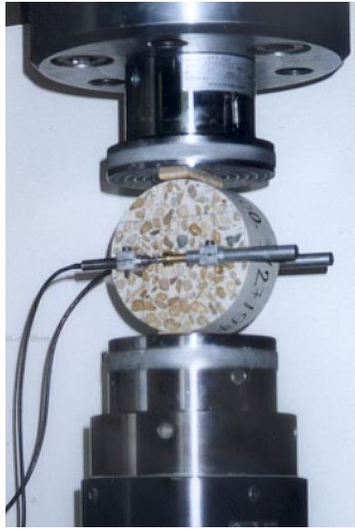
Figure 1: Brazilian splitting tensile test setup.
