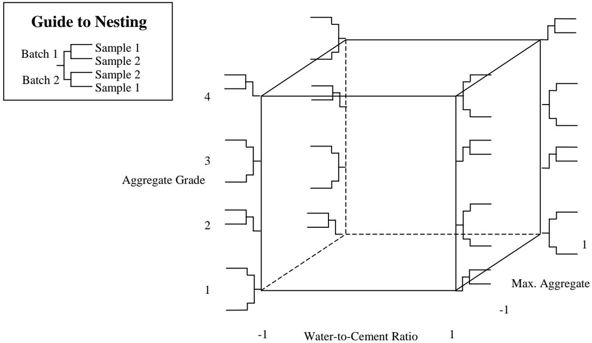
Figure 5. Split Factorial Design for the Concrete Permeability Experiment.
